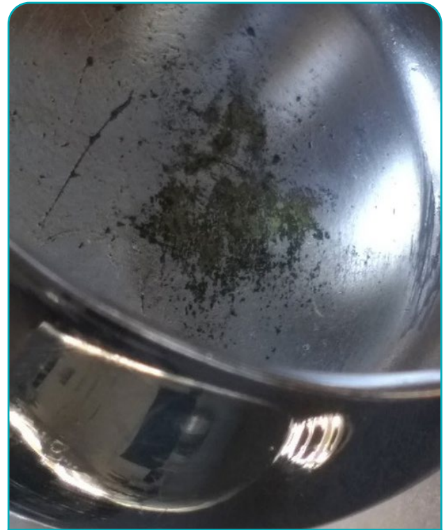
This is corrosion and this cannot be polished but would need to be replated
